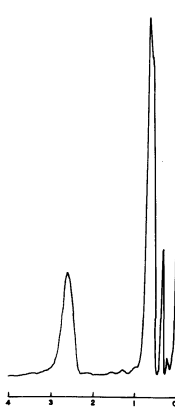
FIG. 1. Typical gas chromatogram of the reaction product after removal of polymers by column chromatography. The peak eluting at approximately 2.3–3.0 min. represents the Diels-Alder adduct. Those eluting before 1.0 min. are fatty acid methyl esters.
